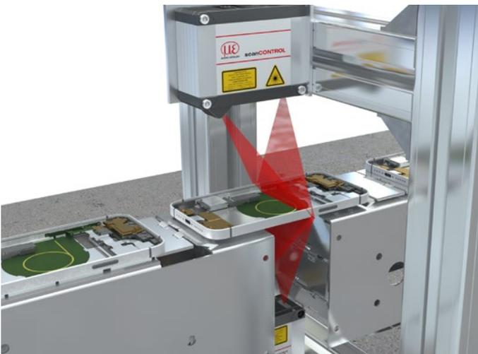
Thickness of smartphone carrier plates
