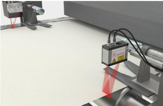
Paper web monitoring and width measurement with two sensors
