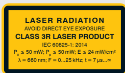
Fig. 8 Laser label and laser warning sign LLT30xx-200
