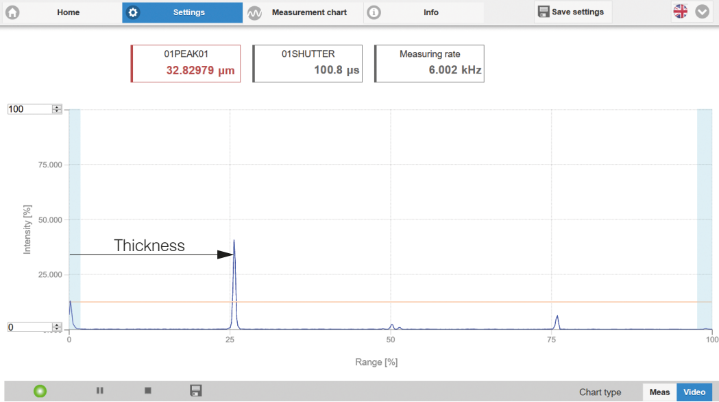
Fig. 7.2: Website FFT signal (thickness measurement)
