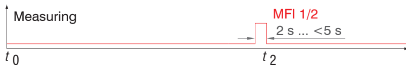
Fig. 6.18: Flowchart for resetting Zeroing/Mastering (Multifunction button)
