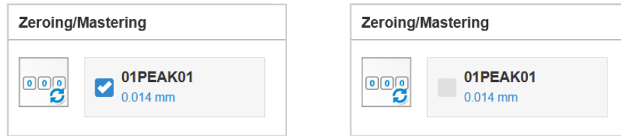
Fig. 6.19: Trigger mastering in the Measurement chart menu by mouse click (left), resetting mastering (right)
