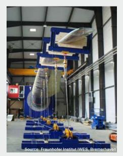
Load tests on rotor blades in a test rig. Draw-wire sensors perform the measuring task.
