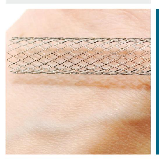
Special feature: Checking the stents for burrs and structural distortions
