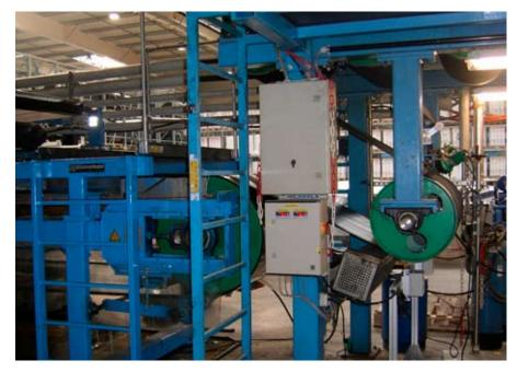
troller. Therefore, only the distance to the rubber surface is required for the layer thickness measurement. Due to its controlled exposure time and measuring rate, the optoNCDT 1700 compensates for weak reflection. In this case, the measuring rate was halved, the exposure time doubled and the measurement filter set to averaging. Due to the extremely high resolution of the optoNCDT 1700, in addition to the distance, the structures in the mesh of the rubber can also be detected.
