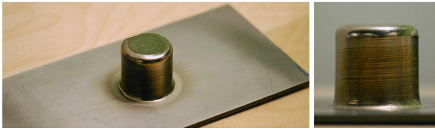
**Fig. 14.** Circular cylinder deposited using iterative learning control.
